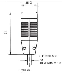
The palm grip B 5 is an actuating element for our multi-axis and single-axis controller. It can also be used as an actuating element for hydraulic drives. Push buttons, rocker switches, e.t.c., can also be fitted to suit appropriate requirements.
