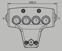
Edition: Sensor installed Pos. 6, Push button installed Pos. 3,4
